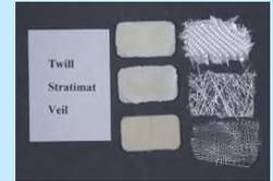
Figure 4. Different E type fiber glass geometries
