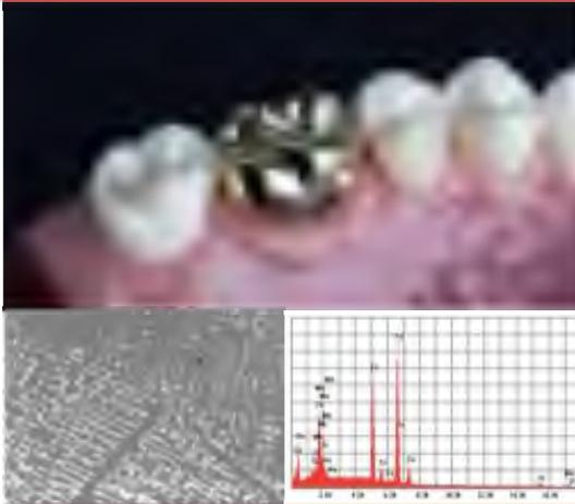
Dental alloy of cobalt-chromium-molybdenum type comprises 47-53 wt.% cobalt, 22-26 wt.% chromium, 4-7 wt.% molybdenum, 0.9-1.2 wt.% silicon, 3-5 wt.% niobium, 0.8-1.1 wt.% ruthenium, 10-14 wt.% zirconium and 2-4 wt.% silver, where the alloy has biocompatible metals comprising molybdenum, zirconium, niobium, silver and ruthenium, and is prepared by elaboration in electric arc furnace in neutral atmosphere.
