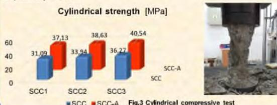
Fig.3 Cylindrical compressive test
