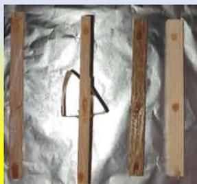
The present invention relates to a composite coating material with consolidating and antimicrobial properties, which provides protection for wood objects with cultural value, based on a solution composed of amorphous silica nanoparticles and an antimicrobial component (composed of hydroxyapatite type, in which calcium has been totally or partially displaced by strontium), dispersed in an aqueous solution of polyvinyl alcohol.
