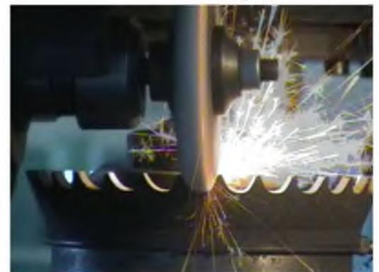
The scheme of the process for machine processing of precession gear teeth.
