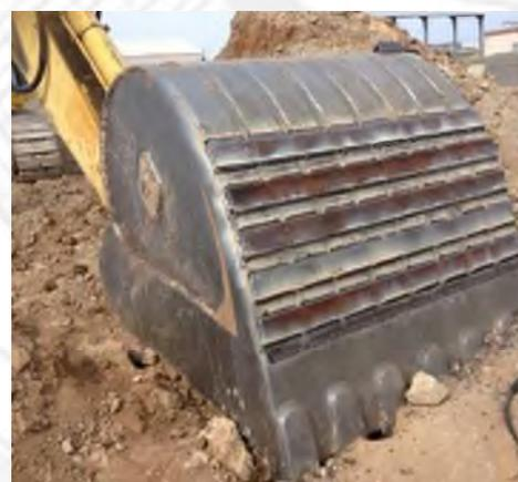
Typical application of wearing plate repair
