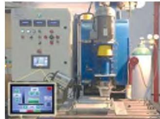
Friction stir welding machine (with inert shielding gas enclosure)
