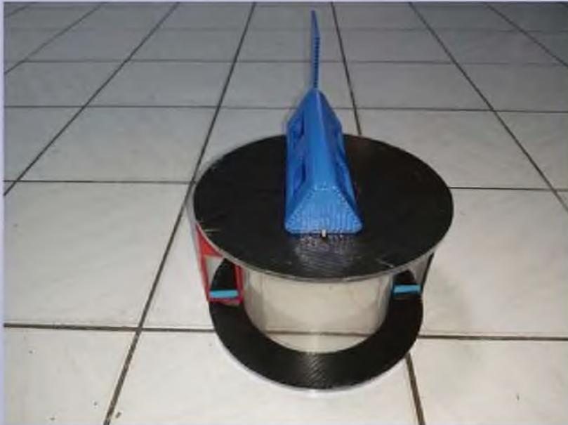
Different from the existing exhaust function of the existing roof ventilation. The ventilator rotates 360° can Turns the vent to the windward side, and bring fresh cool air into the room to regulate the function of reducing indoor temperature. This device can prevent rain or insects from entering the room.
