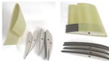
The core of the mold made of laser cut elements from plywood
