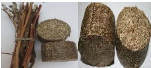
The crop residues (stalks) had moderate gross calorific value of 18.4 MJ/kg, the briquettes have specific density 916 kg/m<sup>3</sup>, were very solid and were not cracking.
