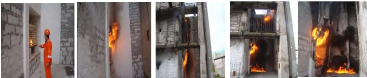
Ignition of the thermal load and the phenomenon of fire propagation at height
