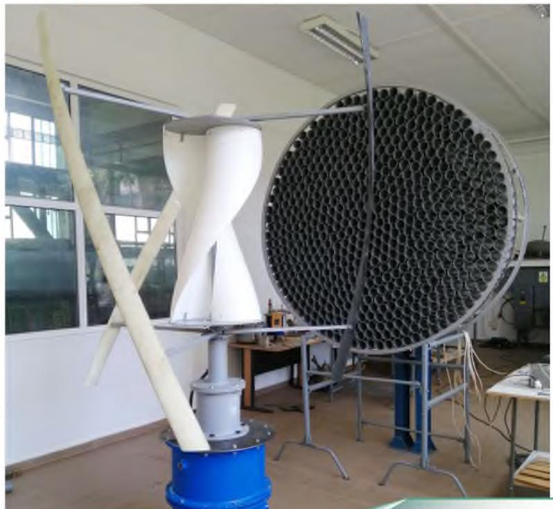
Combination with one rotor the high solidity (Savonius concept) and high tip speed ratio (Darreus concept) permit automatic starting-up the external rotor and increased efficiency in region with low wind potential.
