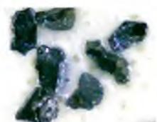
POLYURETHANE NANOCOMPOSITE FLOOR COAT WITH CARBORUNDUM X 20
