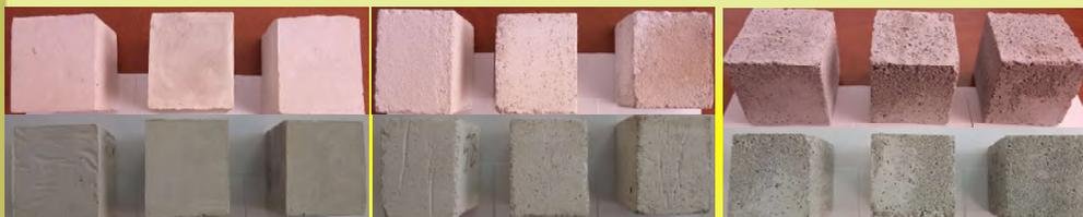
Plaster material treated twice with solvent (left), solution S1 (center) and solution S2 (right), before (up) and after freezing / thawing tests.
