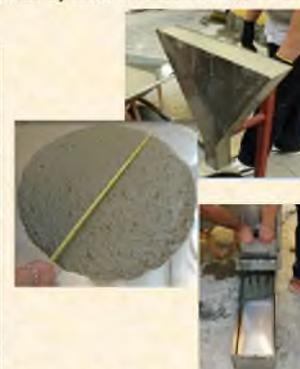
Fig.1 Testing SCC workability
